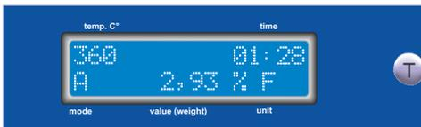
Weigh the sample, pivot the radiator above it, the measurement starts automatically and ends when the weight is constant. Ground moisture is measured using the bright radiator, the **crystal water** is determined using the quartz radiator.
