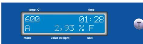
Weigh the sample, pivot the radiator above it, the measurement starts automatically and ends when the weight is constant
